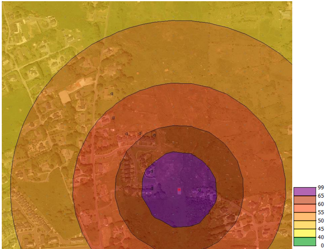
Figure 10.10 Construction phase L_{Aeq\ 1\ h} levels – likely worst case scenario – zone 2
